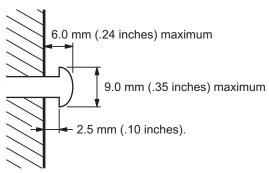
If possible, mount the unit to concrete, masonry, a wooden stud, or some other very solid wall material. Use anchors if necessary (for example, if you must mount the unit on drywall).
